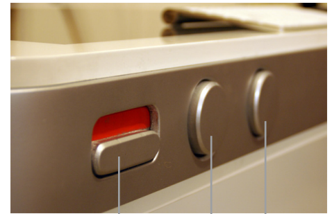
Main Power switch
